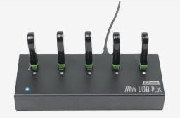
Insert the blank drive into the target ports. When the green light is on, the machine has detected it. When the green light flashes, it starts to copy automatically.
