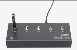
Insert the flash drive with the data to be copied into the Source port. When the green light is on, the machine has detected it. When the green light flashes, it indicates that it starts working.
